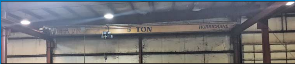
5 Ton & 2 Ton x 40' Approx. Span Brehob Single Girder Top Running Overhead Bridge Cranes
