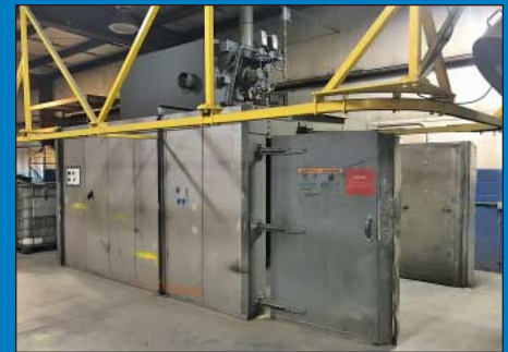
7' x 12' x 6' H Approx. Despatch Model PSC3-66S-1C Drive-In Natural Gas Batch Oven
